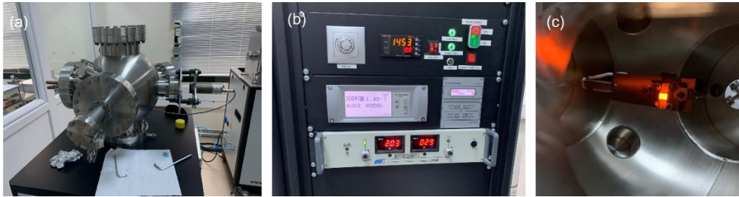
Figure 3.2. a) Ultra-high vacuum epitaxial graphene growth set up b) control panel and c) graphene growth at 1350 °C
