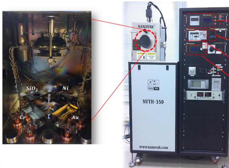
Figure 3.3. Thermal evaporation system for SiO 2 deposition
