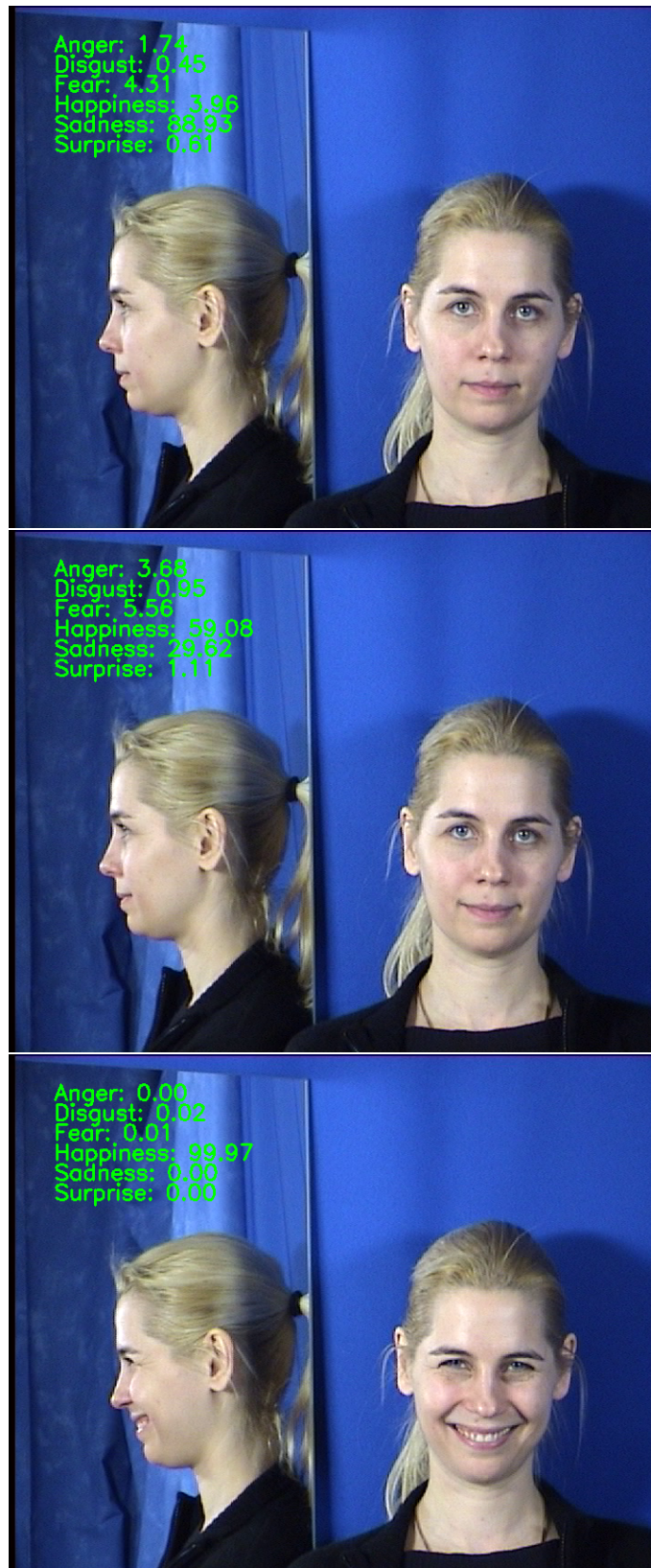
Figure 2.9: Real time prediction results. First frame is taken in between neutral and onset phases. Second frame shows onset phase where facial expression is started. Third frame shows apex phase where emotion is predicted with 99.97% accuracy. Image sequence is taken from MMI dataset (Source: Pantic et al., 2005)
