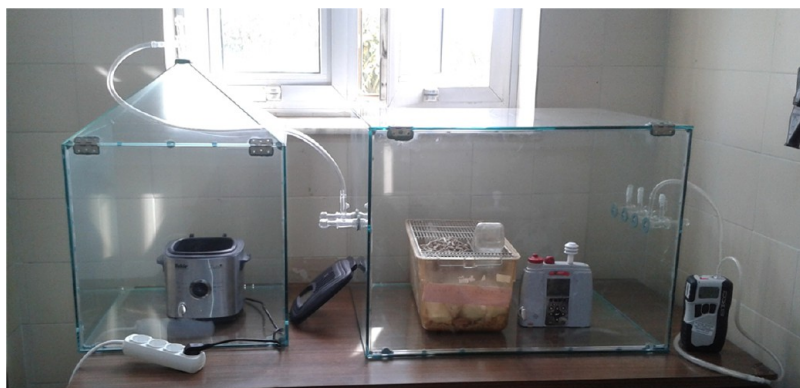
Figure 1. Glass exposure chamber custom-built for the experiment.
