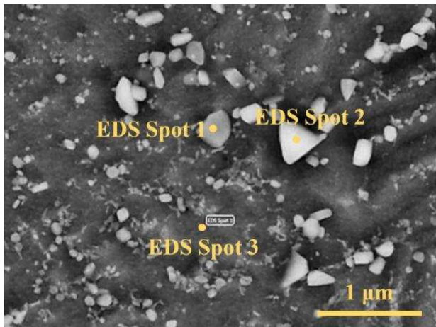
Fig. 7 – SEM image of the SHT1160-treated sample showing the MC type carbides.
