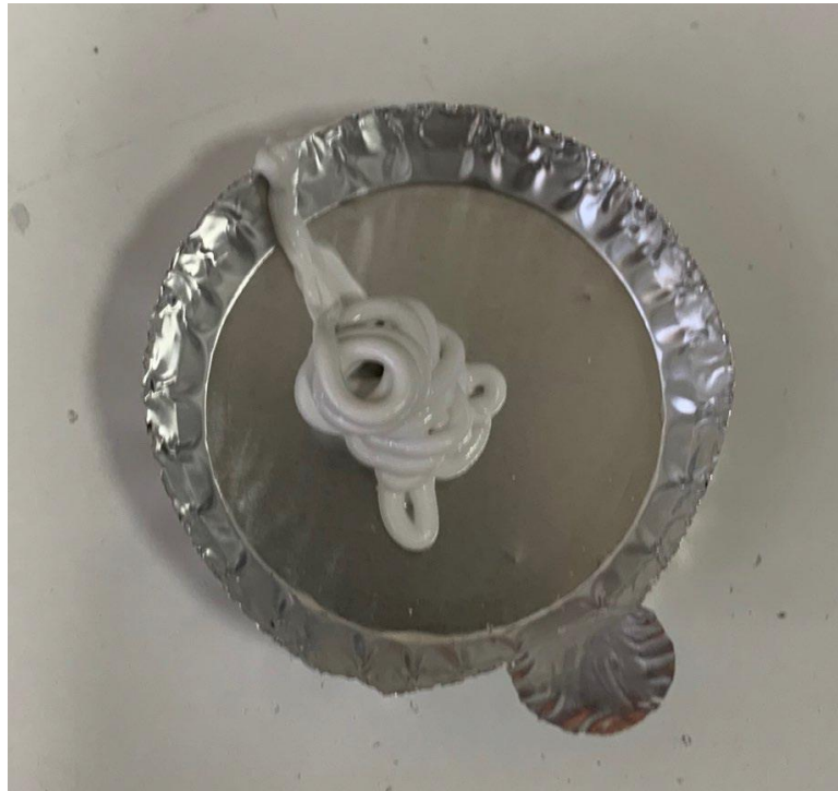
Figure 90. The filament formed as a result of the extrusion test (12.2 gr c3a 1.525 gr marble powder 1.525 gr quartz 5 gr 3.17 hec 5 gr 4m MgSO 4 L/D 15 2mm nozzle 15 mm/min).
