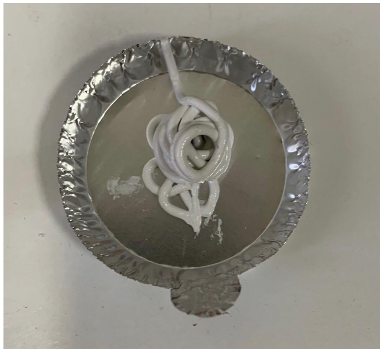
Figure 89. The filament formed as a result of the extrusion test (12.2 gr c3a 1.525 gr marble powder 1.525 gr quartz 5 gr 3.17 hec 5 gr 4m MgSO4 L/D 15 2mm nozzle 10 mm/min).
