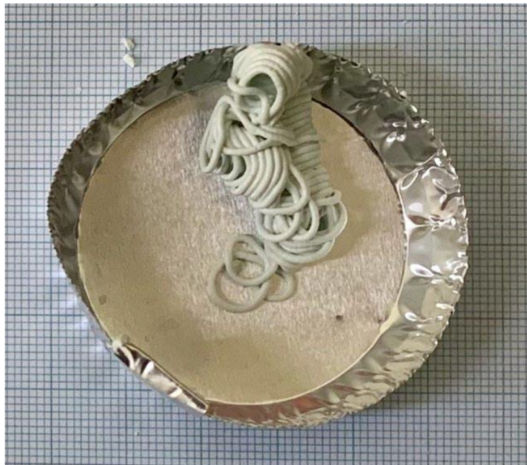
Figure 102. The filament formed as a result of the extrusion test (9.6 gr c3s 1.2 gr quartz 1.2 gr marble powder 3gr 2.5 wt hec 2gr 2M GA 1 gr peg 400 L/D 20 1mm 5 mm/min).
