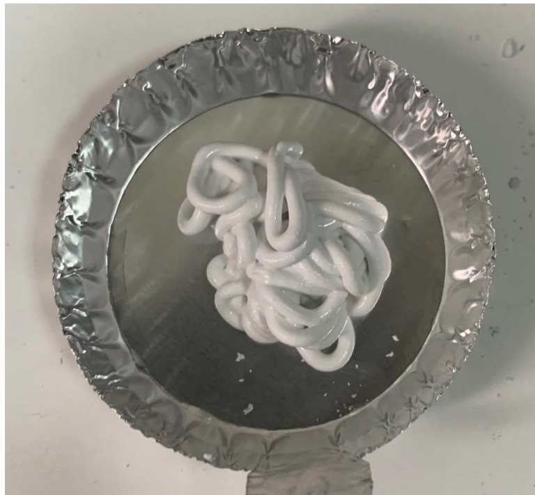
Figure 95. The filament formed as a result of the extrusion test (12.2 gr c3a 1.525 gr marble powder 1.525 gr silica gel 2 gr peg 400 4 gr 3.17 hec 4 gr 4m MgSO4 L/D 15 2mm nozzle 15 mm/min).
