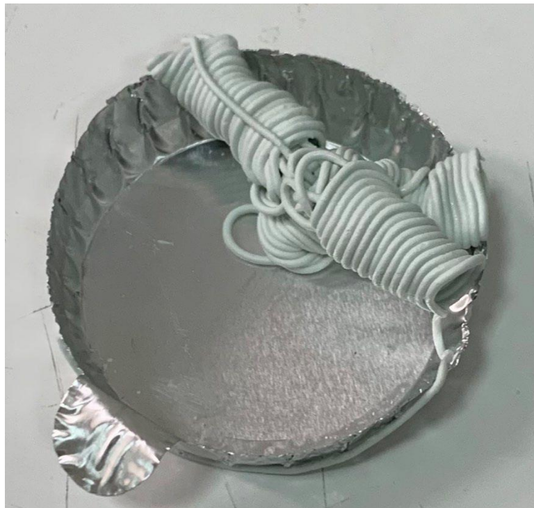
Figure 104. The filament formed as a result of the extrusion test (9.6 gr c3s 1.2 gr quartz 1.2 gr marble powder 3gr 2.5 wt hec 2gr 2M GA 1 gr peg 400 L/D 10 1mm nozzle 10 mm/min).
