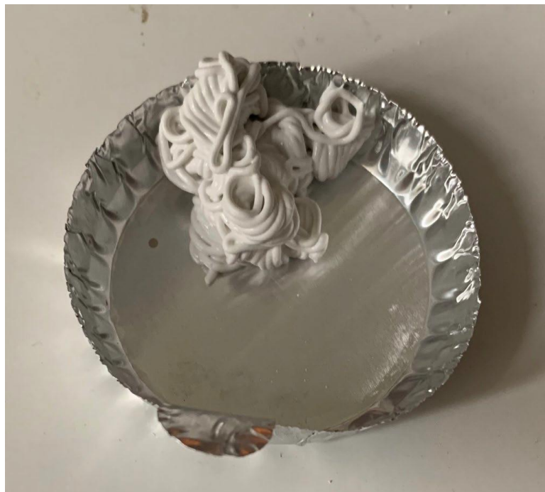
Figure 91. The filament formed as a result of the extrusion test (12.2 gr c3a 1.525 gr marble powder 1.525 gr quartz 5 gr 3.17 hec 5 gr 4m MgSO 4 L/D 20 15 mm/min).
