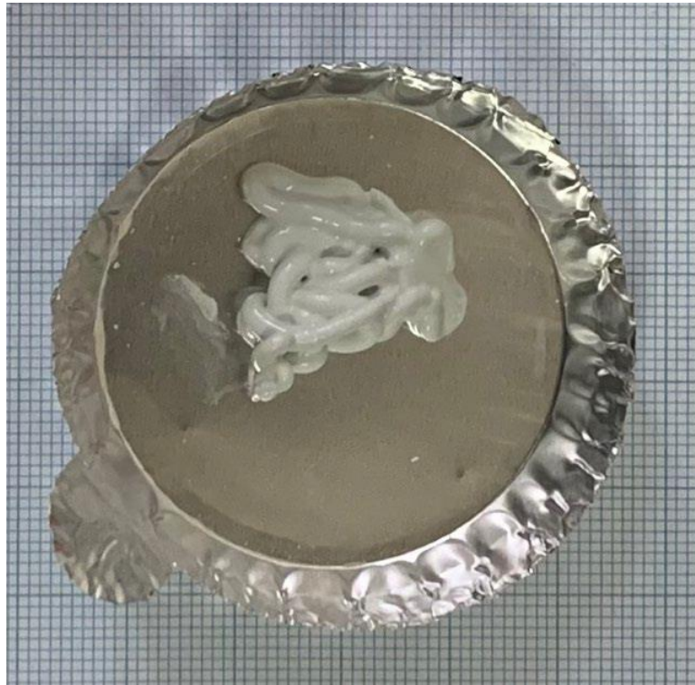
Figure 103. The filament formed as a result of the extrusion test (9.6 gr c3s 1.2 gr quartz 1.2 gr marble powder 3gr 2.5 wt hec 2gr 2M GA 1 gr peg 400 L/D 15 2mm nozzle 10 mm/min).
