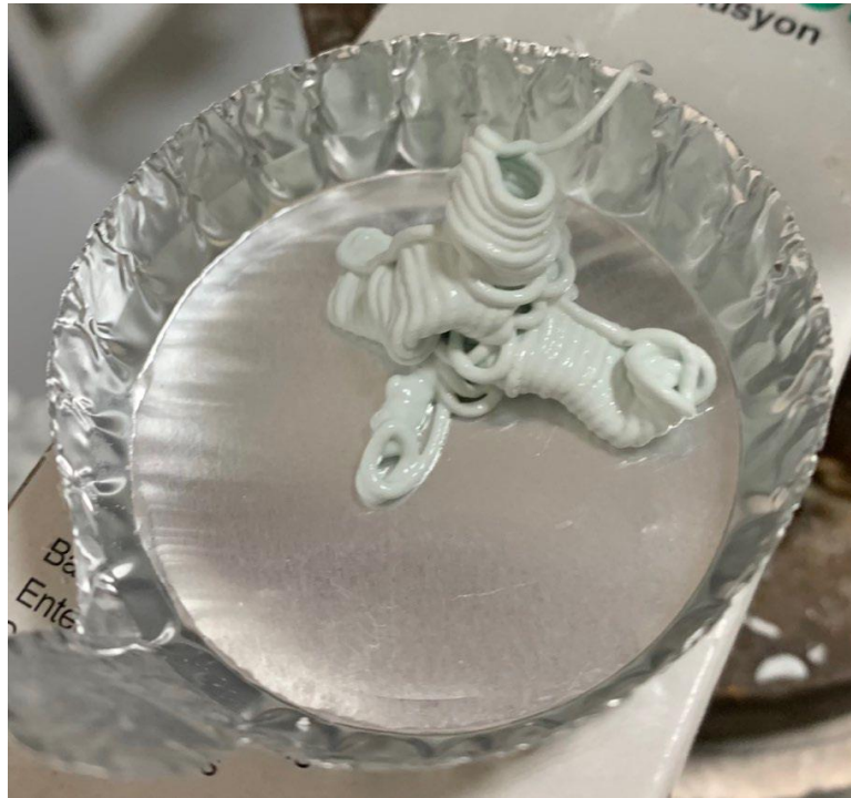
Figure 101. The filament formed as a result of the extrusion test (9.6 gr c3s 1.2 gr quartz 1.2 gr marble powder 3gr 2.5 wt hec 3gr 2M GA L/D20 1mm 10 mm/min)
