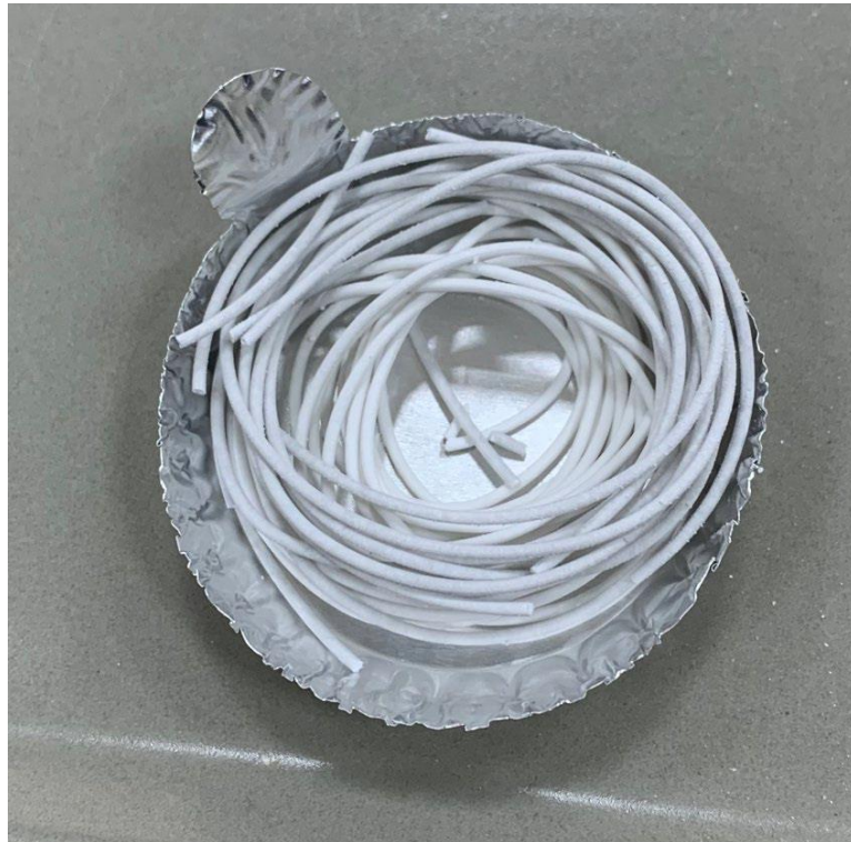
Figure 92. The filament formed as a result of the extrusion test (12.2 gr c3a 1.525 gr marble powder 1.525 gr quartz 2 gr 0.1 M trisodium citrate 4 gr 3.17 hec 4 gr 4m MgSO4 L/D 20 15 mm/min).
