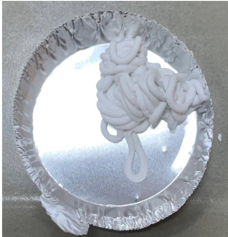
Figure 96. The filament formed as a result of the extrusion test (13.725 gr c3a 1.525 gr marble powder 2 gr peg 400 4 gr 3.17 hec 4 gr 4m MgSO 4 L/D 15 2mm nozzle 10 mm/min).
