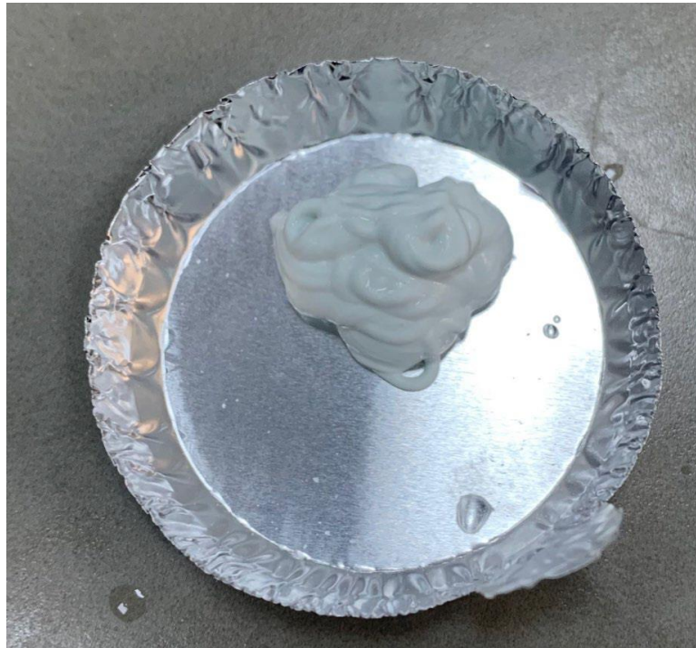
Figure 98. The filament formed as a result of the extrusion test (12gr c3s 6 gr 2.5 hec L/D 20 10 mm/min).
