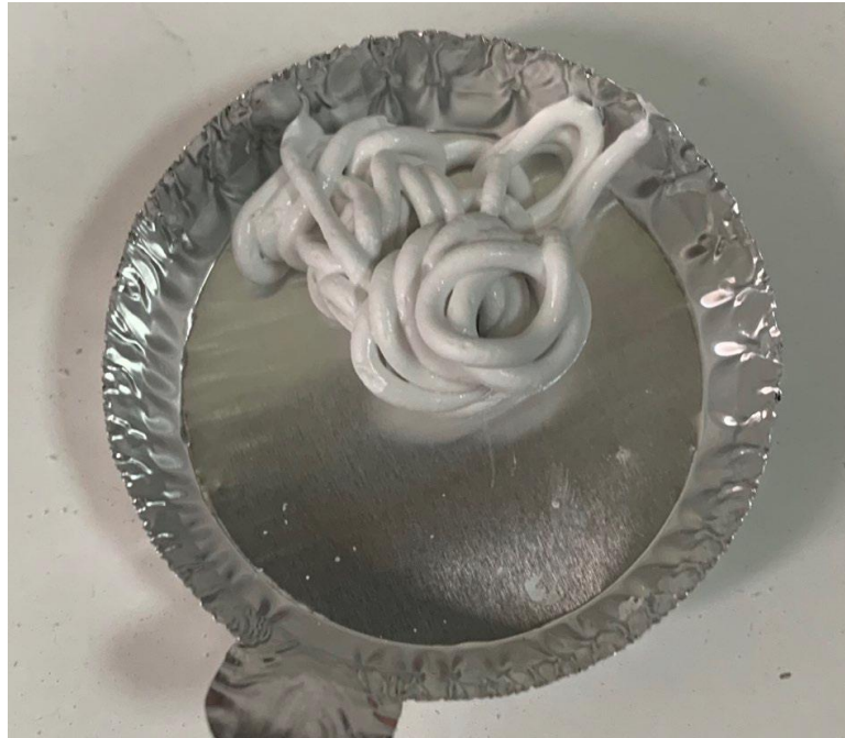
Figure 94. The filament formed as a result of the extrusion test (12.2 gr c3a 1.525 gr marble powder 1.525 gr silica gel 2 gr peg 400 4 gr 3.17 hec 4 gr 4m MgSO4 L/D 15 2mm nozzle 10 mm/min)
