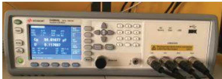
Figure 1.26. The LCR meter (KEYSIGHT, E4980AL) that can measure impedance, capacitance and dielectric loss of samples between 20 Hz and 300 kHz.
