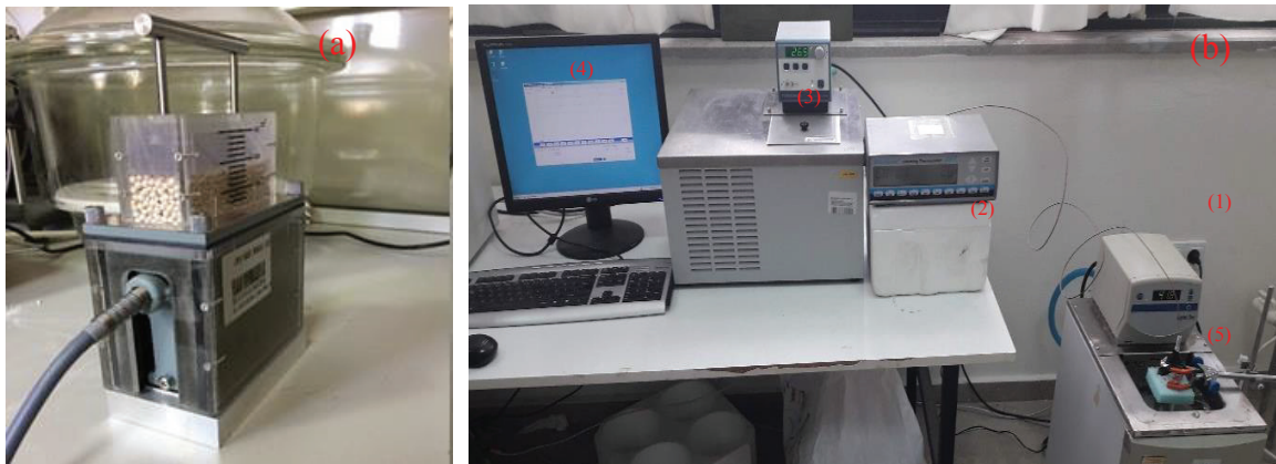
Figure 6.2. Measurement device for thermal conductivity a) Hot wire method b) Heat Source method
