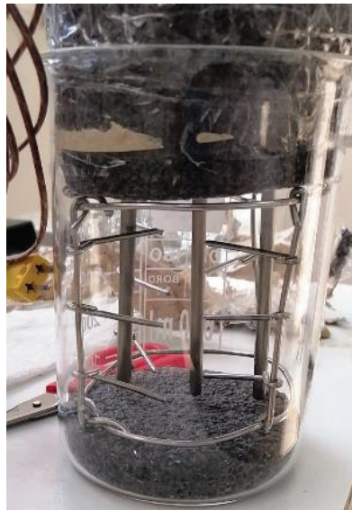
Figure 6.4. Sample holder (SH-2) with three K-type thermocouples
