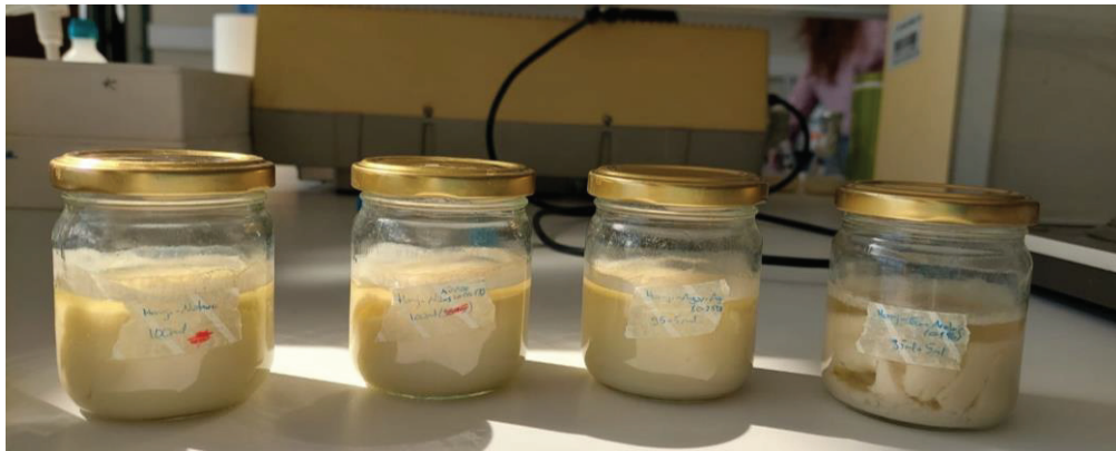
Figure 3.7. Fermented MB: YSL milks in the concept of 3 rd trial (homogenized MB: YSL inoculated by CP pre-culture, with addition of starch, agar-agar, and gum Arabic from left to right)
