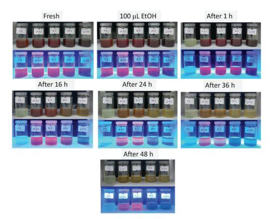
Figure S5.3. Images of CsPbI<sub>3</sub> NCs with varying 4-HBA concentrations after 1 h, 16 h, 24 h, 36 h, and 48 h ethanol exposure under daylight and UV light. The vials are ordered with the concentration of 4-HBA at 0%, 2.5%, 5%, 10%, and 20%, respectively from left to right.
