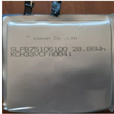
Figure 4.1. 7.5 Ah Pouch Cell (Kokam SLPB705106100)
