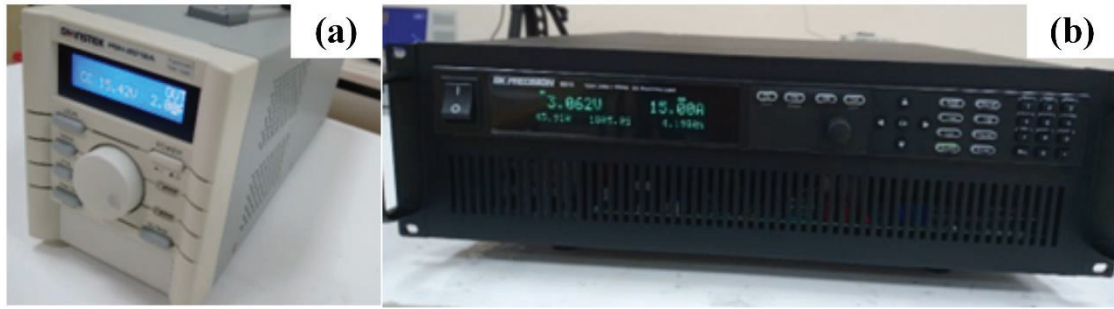
Figure 4.4. (a) Programmable DC Power Supply and (b) Programmable DC Electronic Load
