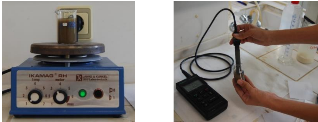
Figure 4.9. a: magnetic stirrer to mix the \text{Ca}(\text{OH})_2 and fine aggregate, b: electrical conductivity analysis by conductivity meter
