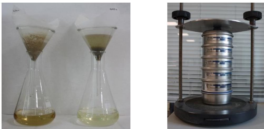
Figure 4.7. a: Filtering of the insoluble parts while washing with distilled water, b: Shaking the aggregates and so eliminating them from series of sieves
