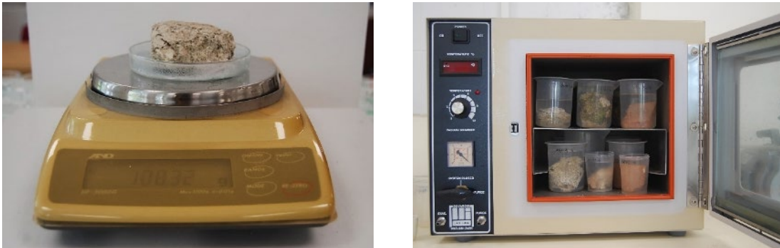
Figure 4.5. a: weighing the dry and saturated samples by precision balance, b: the samples in vacuum oven to saturate them entirely
