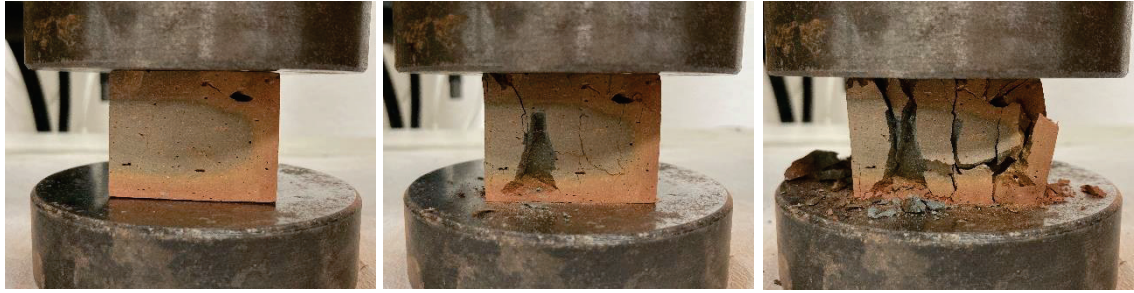
Figure 5.22. The behaviour of AN during the mechanical test
