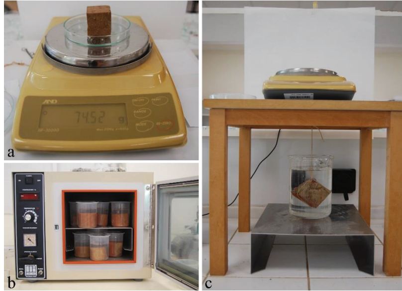
Figure 4.4. a: Weight measurements, b: Samples in vacuum oven, c: Measurements of Archimedes weight
