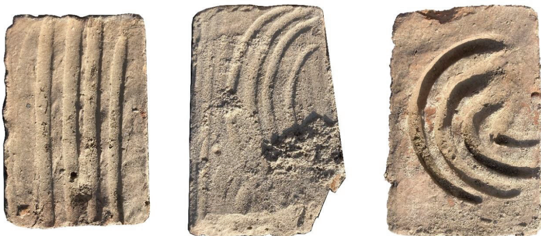
Figure 2.5. In-situ bricks from Anaia Church, Kadikalesi with scratches on the surfaces
