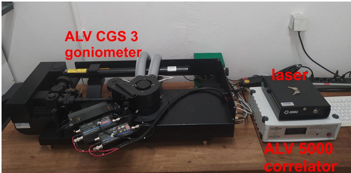
Figure 1.8. Image of ALV multi angular dynamic and static light scattering set-up.
