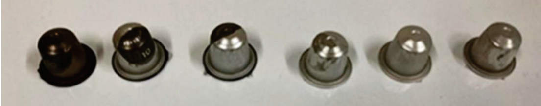
Figure 4.27. Coffee capsule samples after pre-heat treatment at 350, 400, 450, 500, 550, and 600 °C (from left to right).
