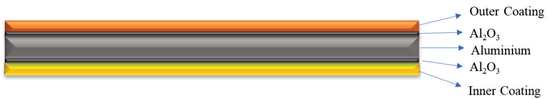
Figure 2.10. Coating layers of beverage can and CC.
