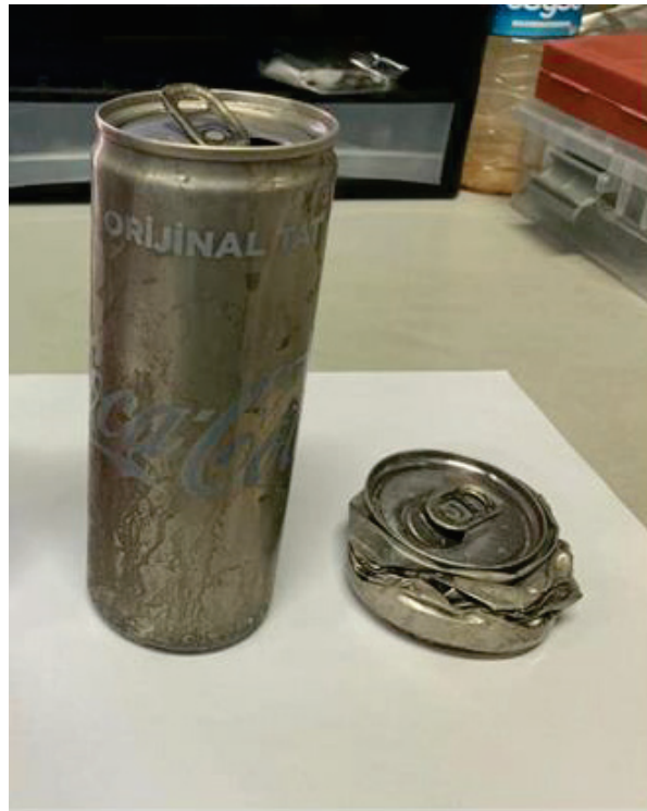
Figure 4.11. Pressed and unpressed UBC samples after thermal pre-treatment.
