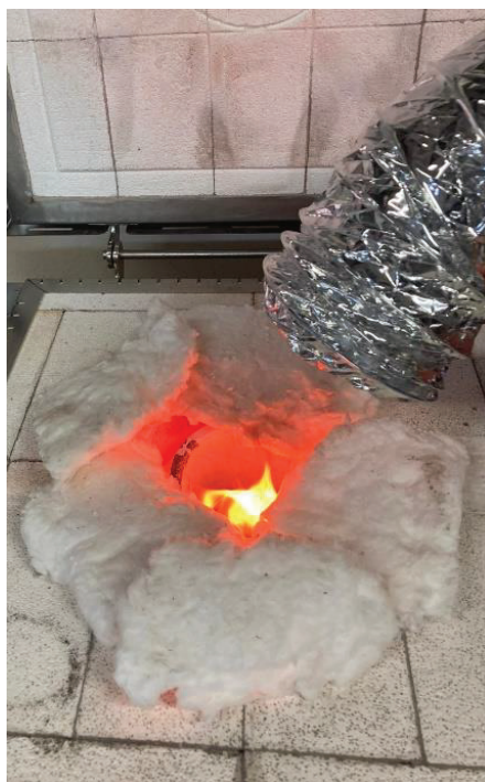
Figure 4.34. Flame observation during the burning of organics on the sample surface.
