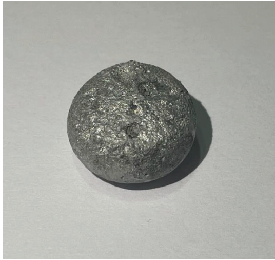
Figure 4.40. Coagulated coffee capsule samples after re-melting under salt flux
