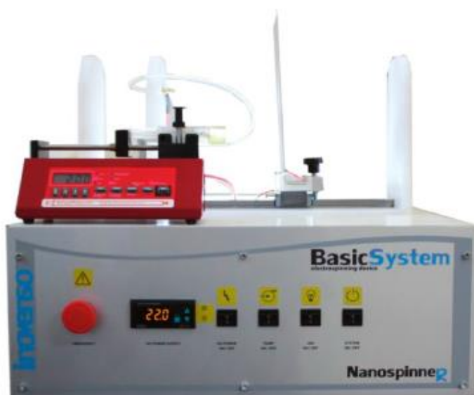
Figure 2.2 Nanospinner basic electrospinning unit (NanoSpinner 1 Electrospinning Equipment - Inovenso Inc. - PDF Catalogs | Technical Documentation | Brochure)
