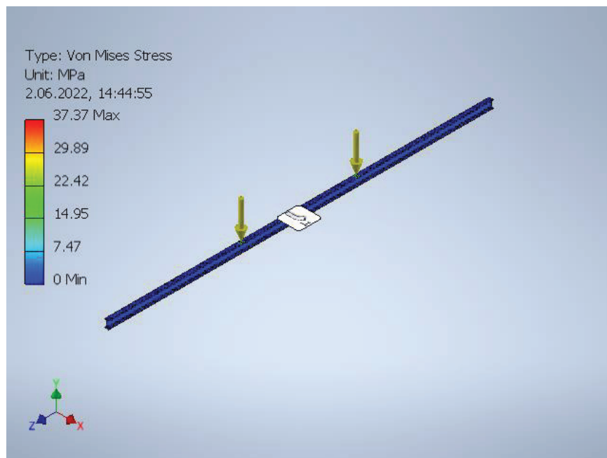
Figure 25. Von Mises Stress Result of the Rail
