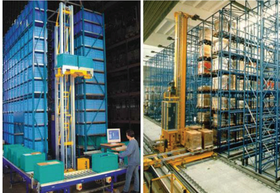
Figure 1. Automated Storage and Retrieval System
