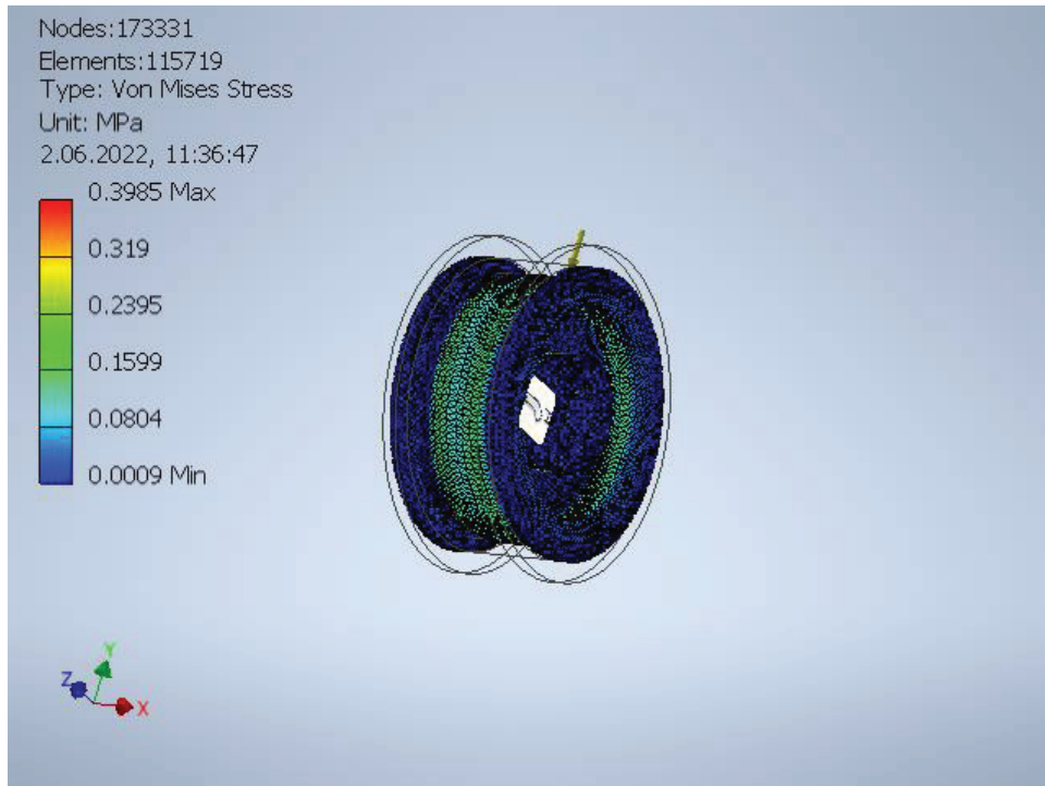
Figure 31. Von Mises Stress Result of the Wheel
