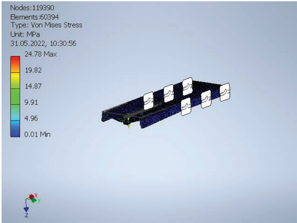
Figure 43. Von Mises Stress Result of the Fork Mechanism-Top Layer
