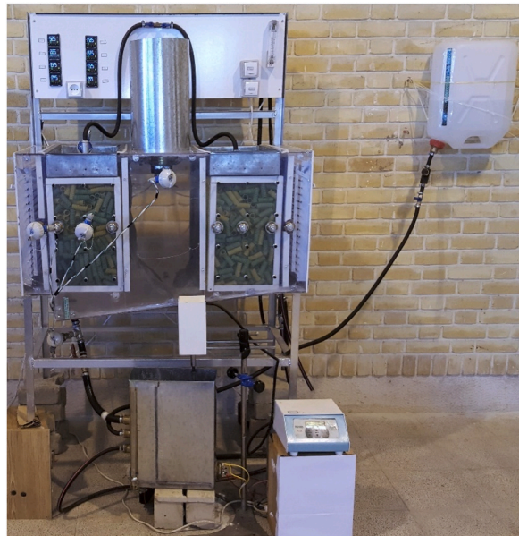
Fig. 6. Exterior view of the assembled experimental cross-flow cooling tower.
