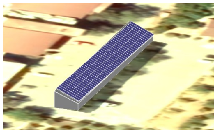
Figure 31: North oriented panel array 3D view
