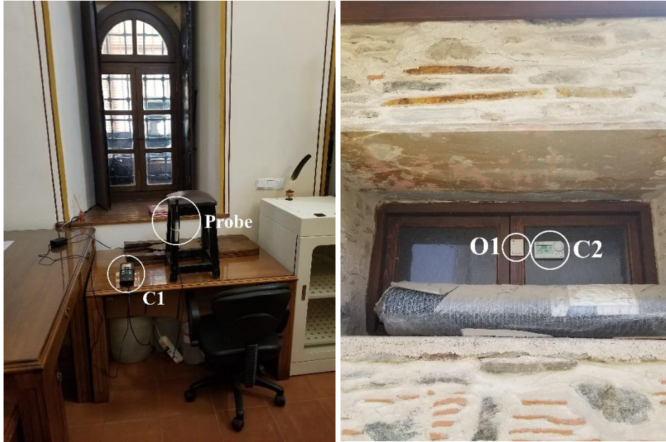
Figure 3.11. CO 2 loggers at their respective locations (left for indoors, right for outdoors)
