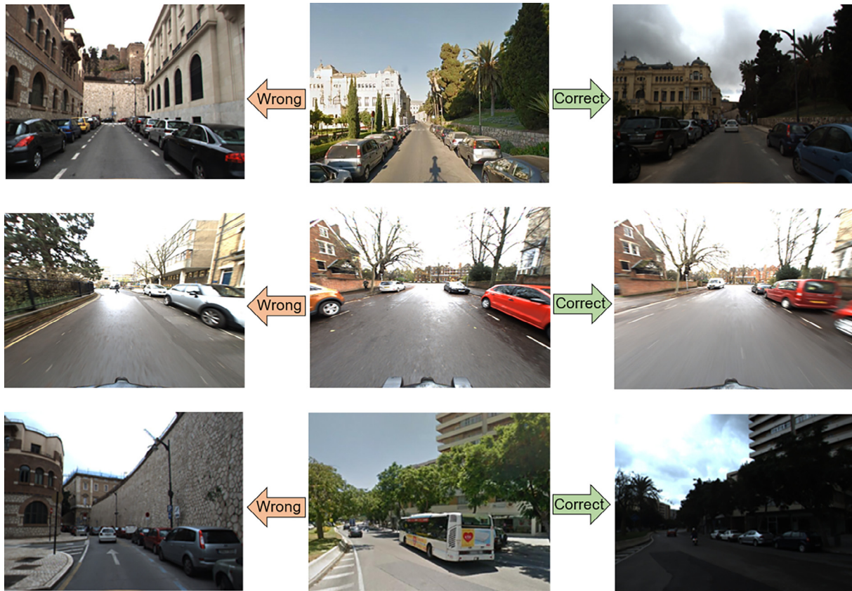
Fig. 11. Superiority of proposed Hybrid-VL method with three sample localization cases from both datasets. RGB image based method LD-VL (left) fails but Hybrid-VL (right) retrieves correct images for a given query (middle).
