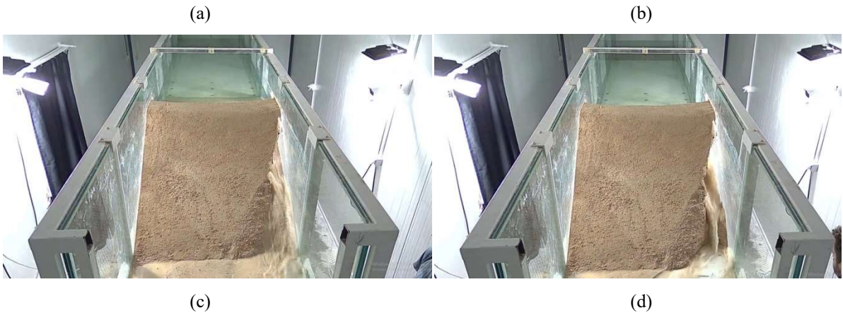
Figure 5. The temporal development of the breach at downstream a) t=0 s, b) t=220 s, c) t=340 s, d) t=680 s
