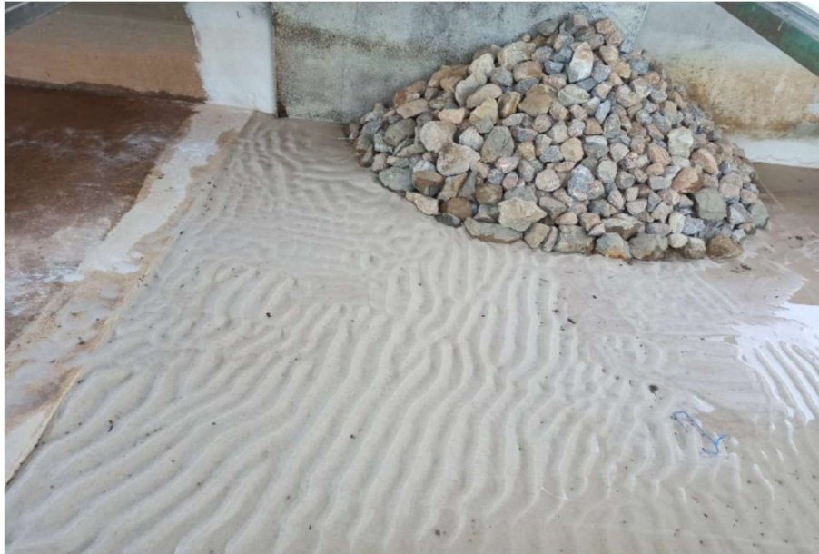
Figure 10. The final state of the breakwater surrounding as a result of experiment 1
