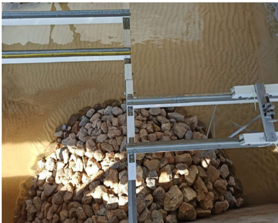
Figure 11. The final state of the breakwater surrounding as a result of experiment 5
