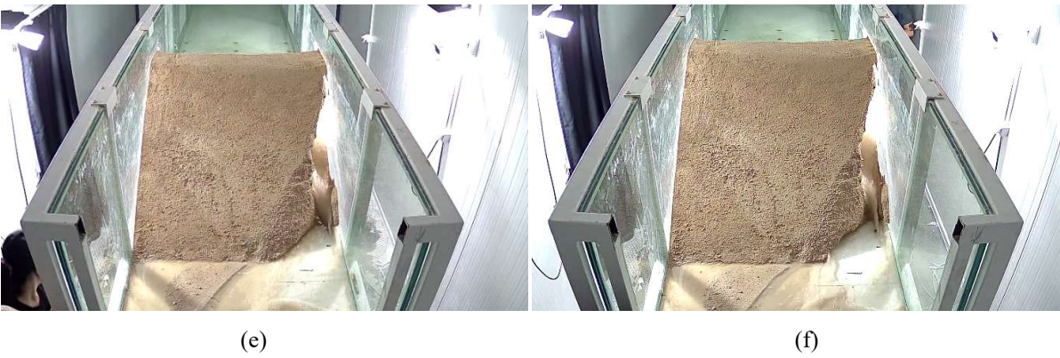
Figure 5. The temporal development of the breach at downstream (continued) e) t=1020 s, f) t=1360 s
