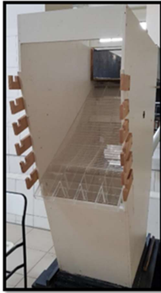
Figure 4. Wooden sockets assembled on intake walls
