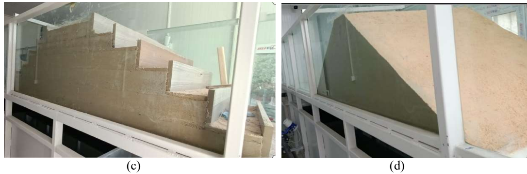
Figure 4. Some construction stages (continued): c) After compaction of the last layer, d) final shape
