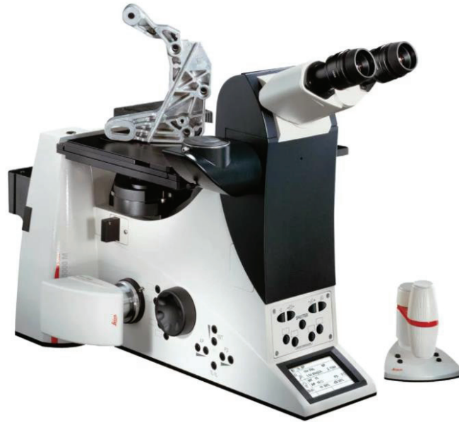
Figure 3.2. Leica DMI5000 model optical microscope is used for examining the samples.
