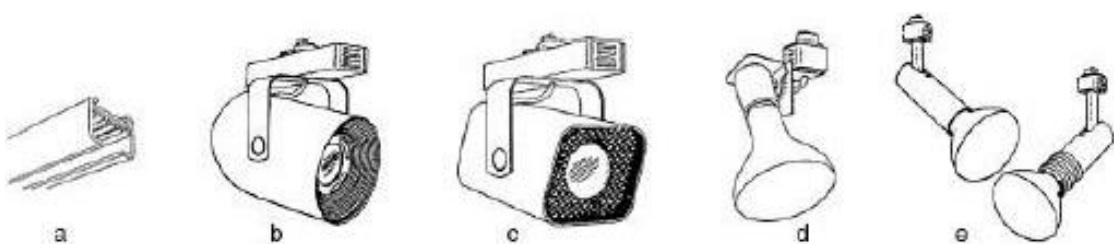
Figure 2.13. Examples of track luminaires: (a) close-up of multicircuit track, (b) and (c) track-mounted luminaires with optical control, and (d) and (e) track luminaires for holding and aiming lamps (Source: IESNA, 2011).
