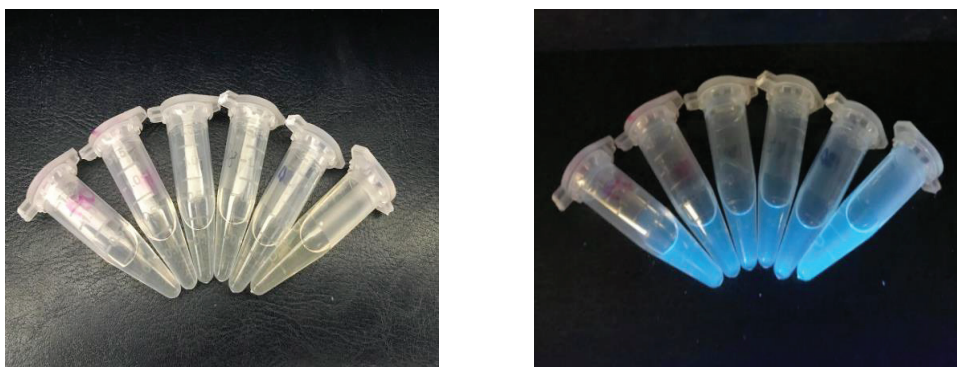
Figure 2.15. The color of the CD solution after 10 hours later under daylight (left) and UV-light (right) from left to right (5h,6h,7h,8h,9h,10h)
