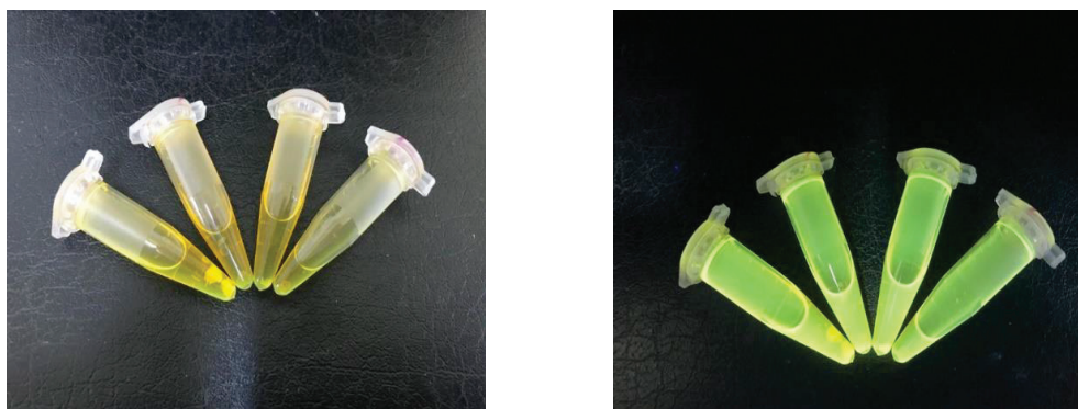
Figure 2.18. After reaction every hour solid particle was diluted with ethanol under daylight (left) and UV-Lamp (right) (2,4,5,6 hours from left to right)
