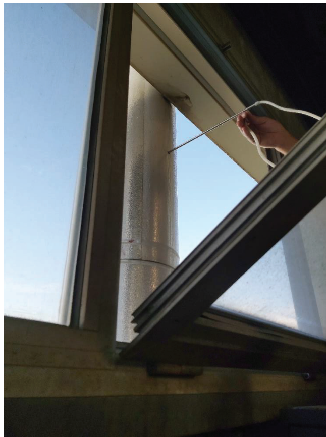
Figure 2.11. Measurement of the pressure differences of the chimney gas to obtain volume flow rate of it
