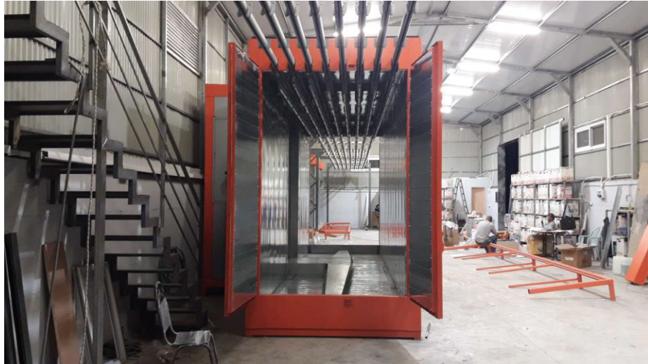
Figure 1.2. Typical industrial drying-curing convection oven / ELECTRON Company Internal Report
