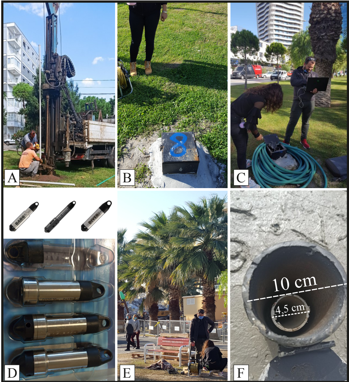
Figure 2. Photos of a) drilling phase, b) final state of the wells c) diver measurement stage, d) divers, e) measurement studies near collapsed buildings after the earthquake, f) well diameter features.
