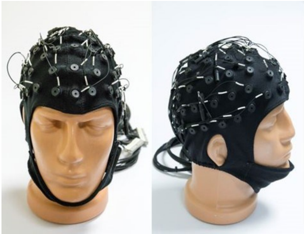
Figure 7. The illustration of 64 electrodes on a head model placed according to 10/10 recording system.
