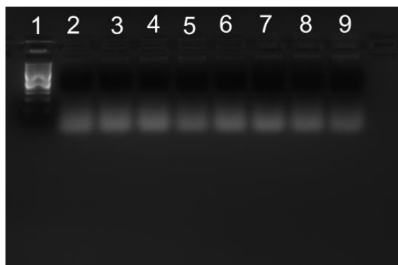
Figure 4.34. Agarose gel electropherogram of star polymer-siRNA complexes, SP1 and SP2, at N/P of 50, incubated at 50% FBS (v/v) for varying times. Lane 1: Marker, Lane 2-5: SP1-siRNA complexes after incubation in serum containing media for 0 h, 2 h, 8 h, and 24 h, respectively. Lane 6-9: SP2-siRNA complexes after incubation in serum containing media for 0 h, 2 h, 8 h, and 24 h, respectively.
