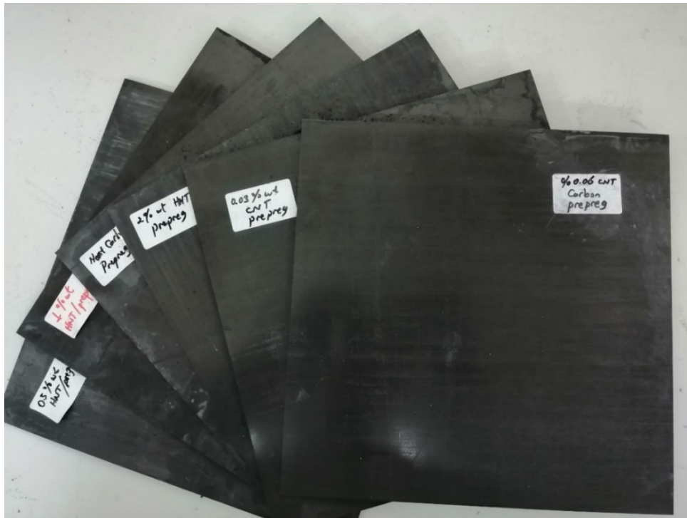
Figure 7.25. Representative image of the manufactured laminates containing various amounts of F-SWCNTs
