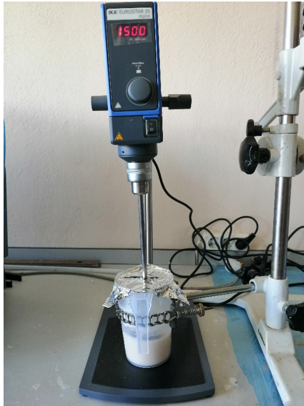
Figure 6.1. The mechanical high-speed mixing setup for preparing neat epoxy resin system
