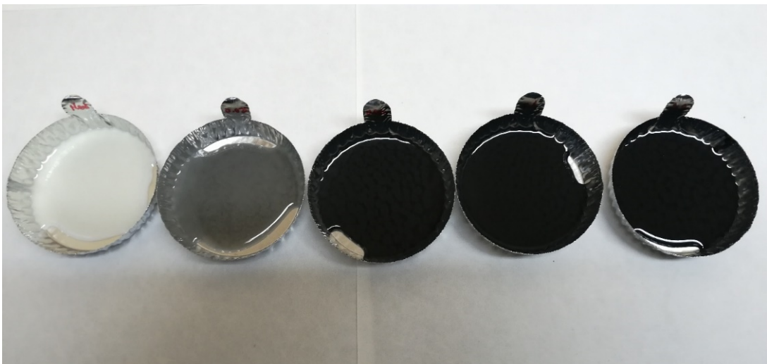
Figure 7.6. The image of functionalized SWCNT (F-SWCNT) /epoxy blends after preparation as presented in the experimental section
