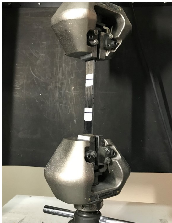
Figure 6.20. CFRP standard tensile test setup
