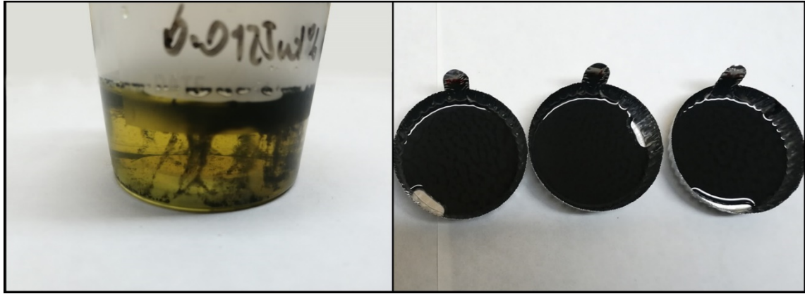
Figure 7.7. Images of pristine (un-modified) and F-SWCNT /epoxy blends after 1-hour preparation stage. (left) Pristine SWCNTs/epoxy, (right) 0.05, 0.1, and 0.2 wt. % functionalized F-SWCNTs/epoxy blends, respectively
