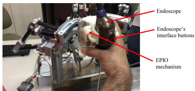
Fig. 8 Endoscope mounted to the NeuRoboScope system via the EPIO mechanism
