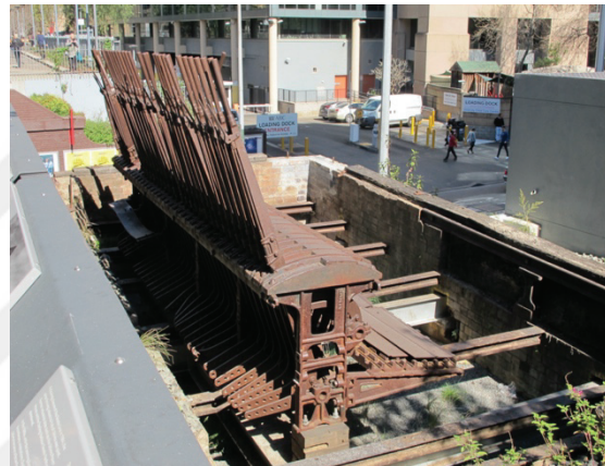
Figure 55. Interlocking machine in the design (Source: https://maas.museum/inside-the-collection/2015/09/03/the-goods-line-then-and-now/ )
