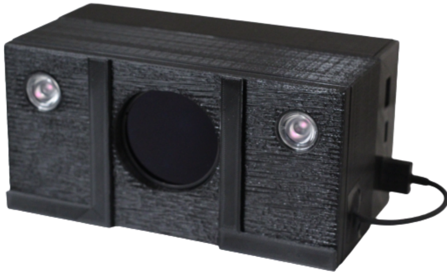
Figure 2.13. Print out of device. LEDs powered by the USB cable coming from the power bank.
