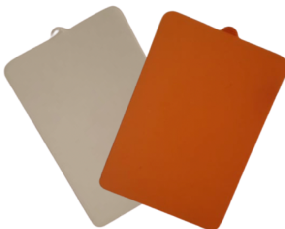
Figure 2.8. Diffusers used to diffuse NIR light. The difference in colors effects the amount of diffused light. The orange diffuses the light more than white (orange was used in the study).
