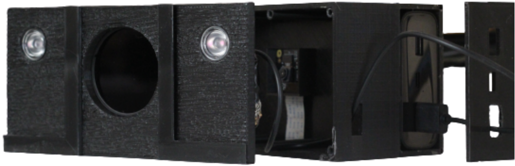
Figure 2.11. The output of all parts of the device. The lid of the camera box holds the LEDs, infrared filters and diffusers. There is a camera module in the holder inside the camera box, and there is a power bank box on the back of the camera box with the power bank that powers the LEDs.
