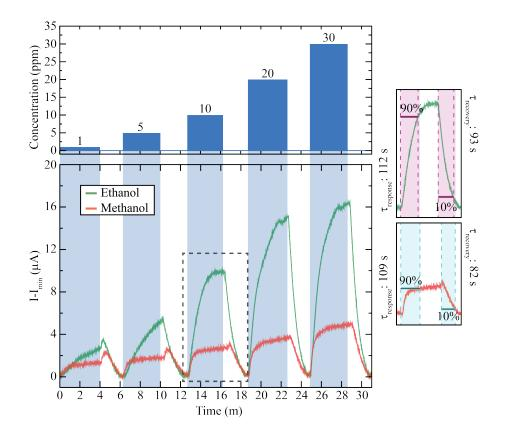
Figure 8.3. (a) Concentration dependent response to methanol and ethanol, displayed with red and green lines, respectively (b) response and recovery times of the methanol and ethanol measurements.
