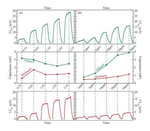
Figure 8.4. Voltage and concentration dependent capacitance of the methanol/graphene and ethanol/graphene systems with corresponding response readout.
