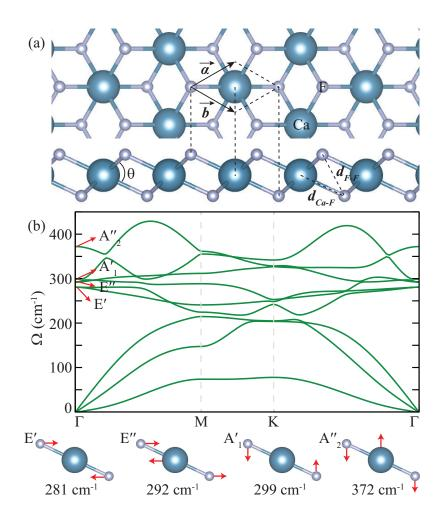
Figure 3.1. (a) Top and side views of 1T-CaF<sub>2</sub>. (b) Phonon dispersion of 1T-CaF<sub>2</sub>. Modes with corresponding frequencies are shown in the inset. Reproduced from Ref.<sup>14</sup> with permission from the PCCP Owner Societies.
