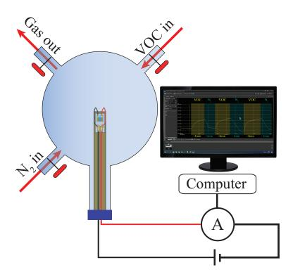
Figure 2.3. Experimental setup for gas sensing application.
