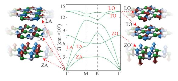
Figure 2.1. Phonon band dispersions and corresponding vibrational modes of h-BN.
