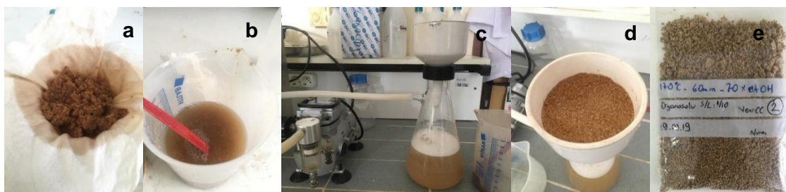
Figure 3.2. Preparation of organosolved solid to the enzymatic hydrolysis.
