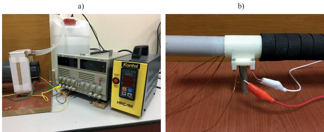
Figure 3.16 Zoom-in pictures of the experimental setup a) control units, b) sample holder
