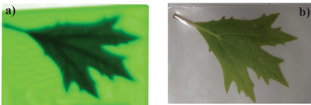
Figure 4.3. a) THz transmission at 0,537 THz and b) visible image of a leaf.
