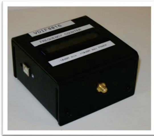
Figure 3.2. VDI 0.5-20 GHz Frequency Counter
