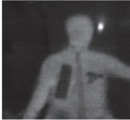
Figure 2.1. A passive THz image of A handgun and a rectangular piece of standard RF anechoic material are concealed under the clothing (Shen et al. 2008).
