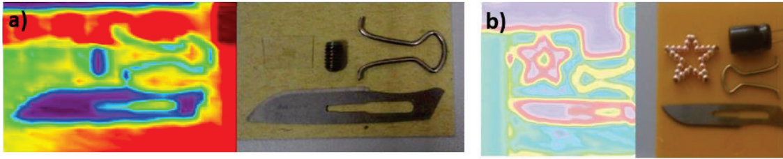
Figure 4.2. Terahertz images taken at a) 0.537 THz b) 0.600 THz.
