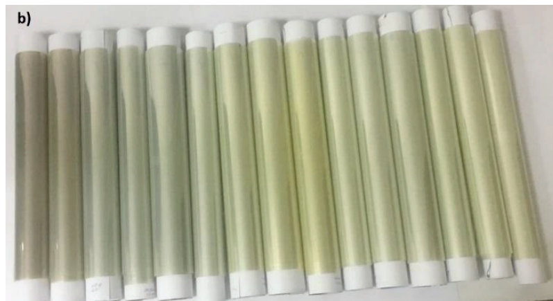
Figure 3.11. a) Schematic representation of our large area magnetron sputtering coating system, b) ITO deposited flexible Polyethylene terephthalate (PET) films (7 cm rolled, 40 cm width, 10 m long for each process parameter).
