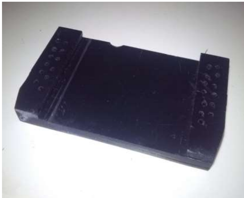
Figure 3.9. CCD camera slider bed
