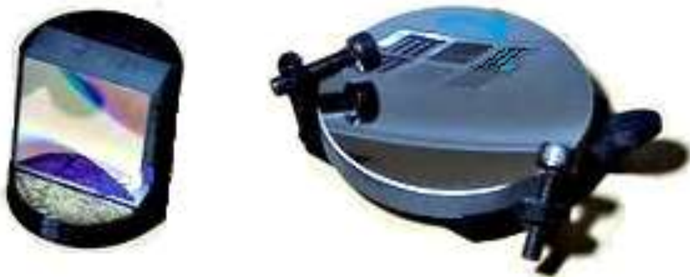
Figure 3.3. Grating and focusing mirror and their holders. Holders are printed by 3D printer.
