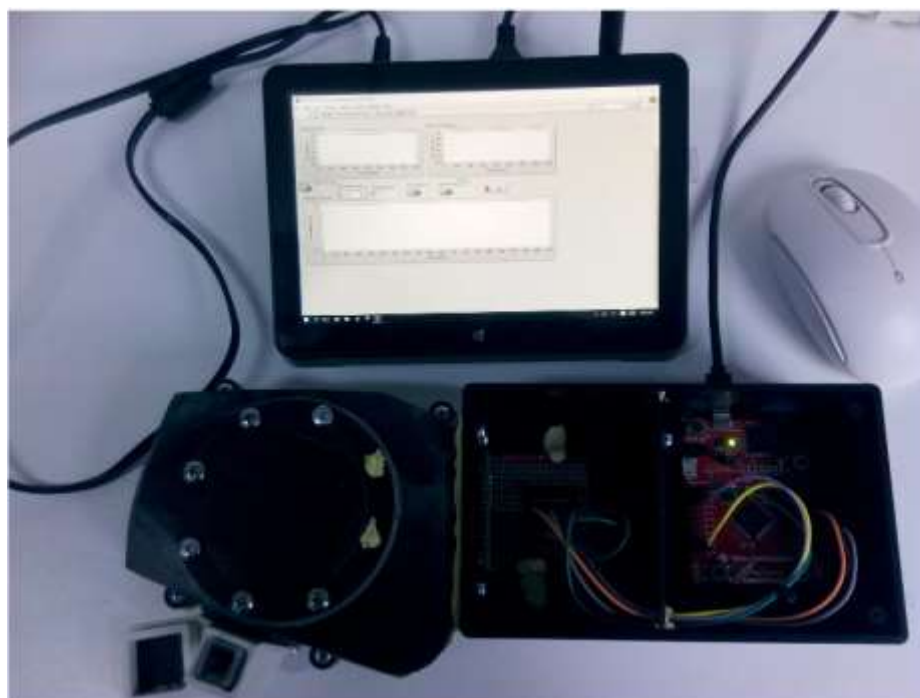
Figure 3.11 Completed set-up of our Prototype Spectrometer.
