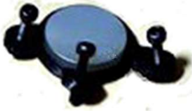
Figure 3.2. Collimating mirror and holder. Holder is printed by 3D printer.
