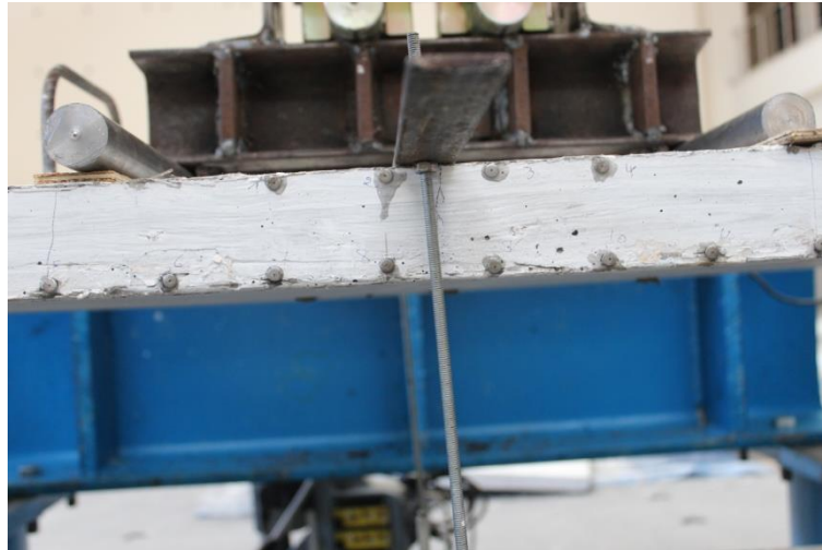
Figure 32: Beads for the four-point bending test.
