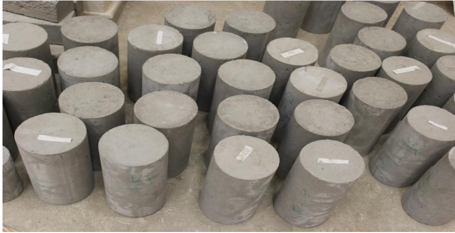
Figure 34: The cylinders ready to be tested.
