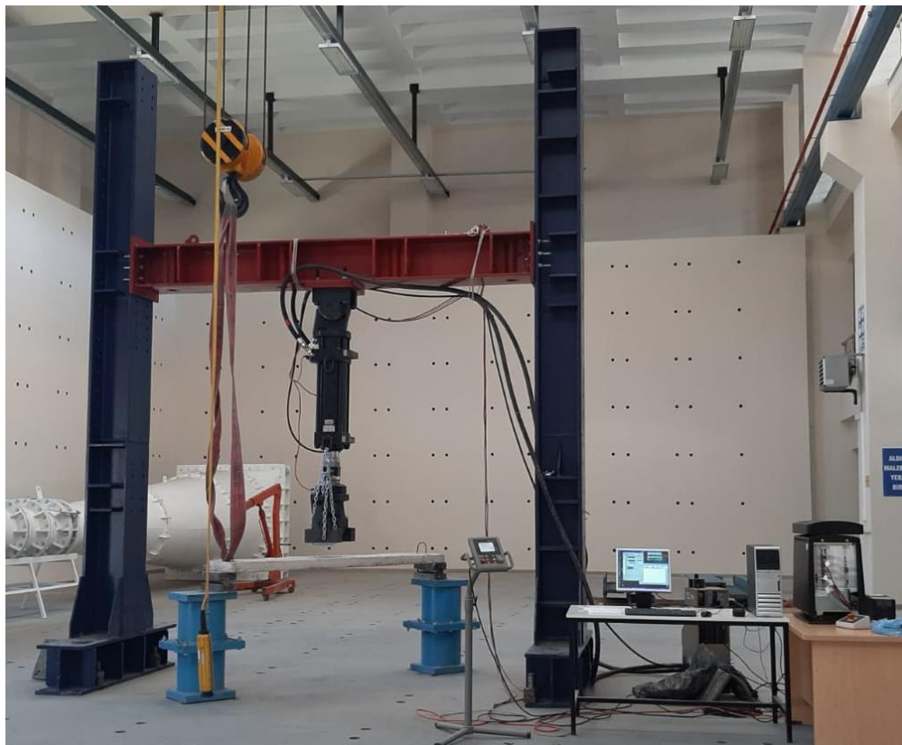
Figure 22: Bending test mechanism
