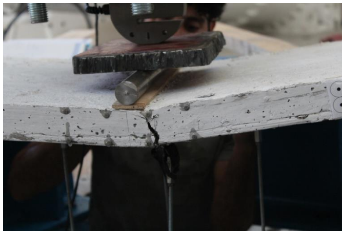
Figure 48: Final view of SA3+PVA after testing
