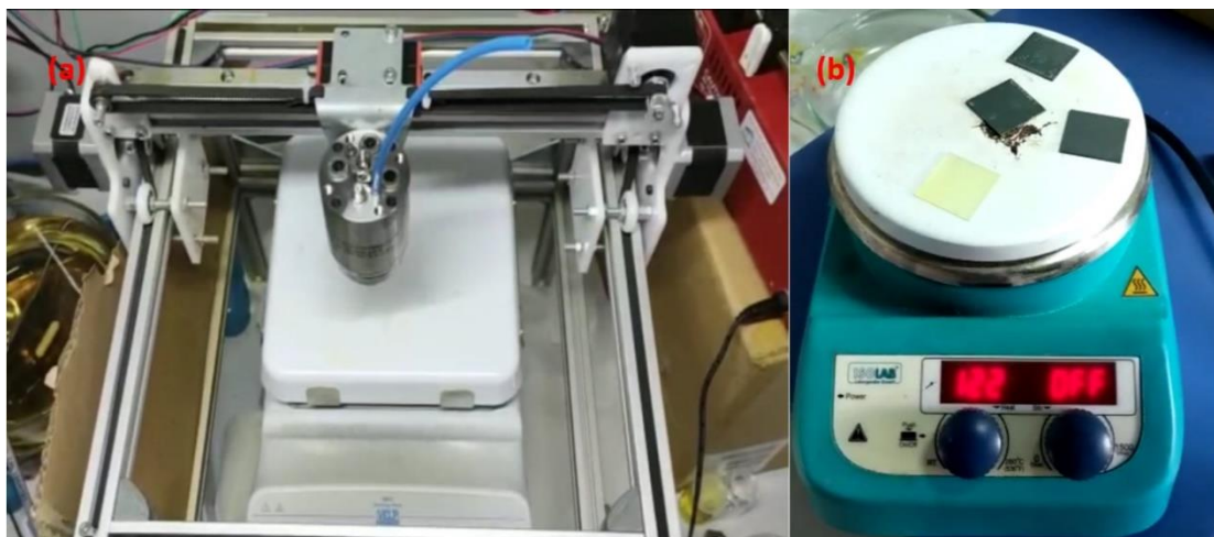
Figure 3. 4 Hot plates used in the experiment, (a) to control the substrate temperature, (b) to anneal our samples.
