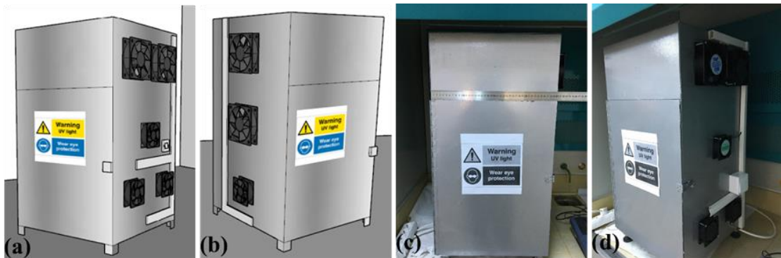
Figure 2. 1. The 3D Autocad drawings (a & b), and the photographs of UV lamp cabin system (c & d).
