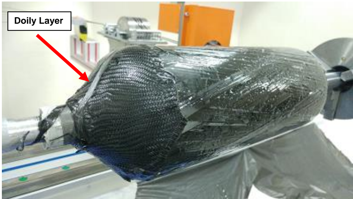
Figure 3.25. Doily layers placed over the boss region during the filament winding process.
