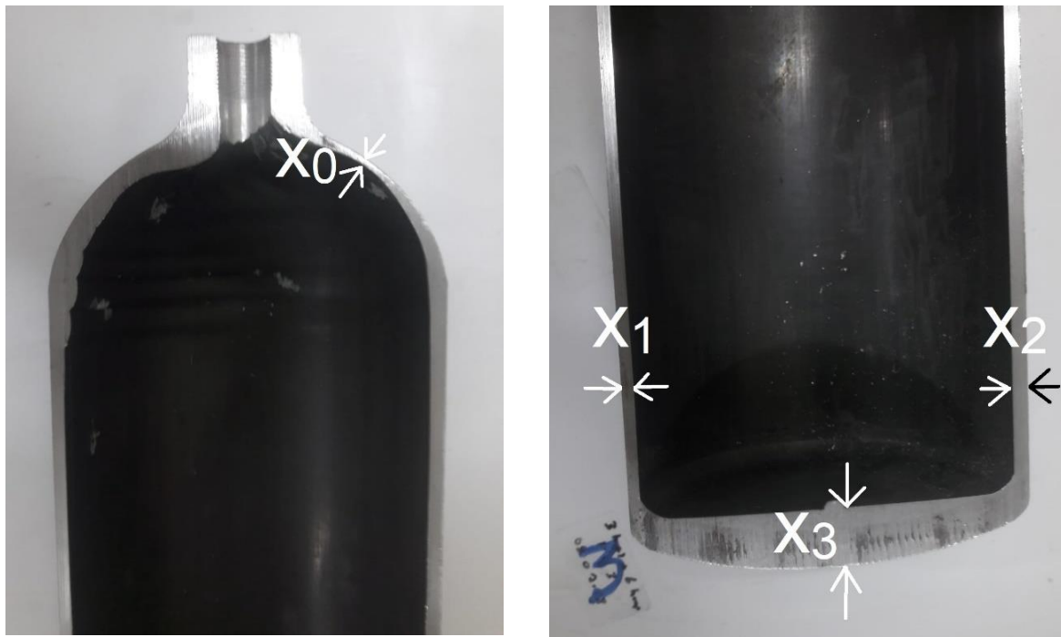
Figure 3.23. Cross section of aluminum liners manufactured as first try.
