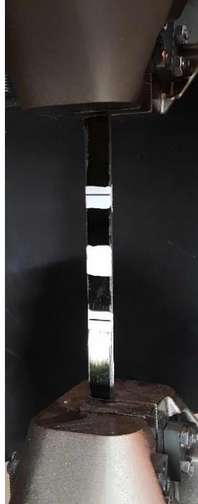
Figure 3.5. Carbon/epoxy tensile test specimen during tensile testing.
