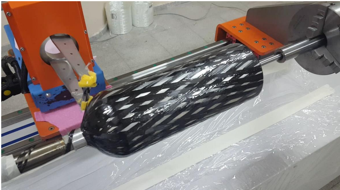
Figure 3.22. A helical layer winding of carbon/epoxy over the aluminum liner.
