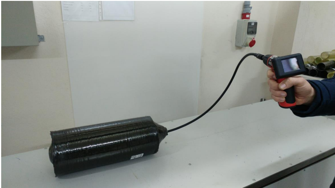
Figure 3.26. Inside wall control of a composite tank by snake cam.
