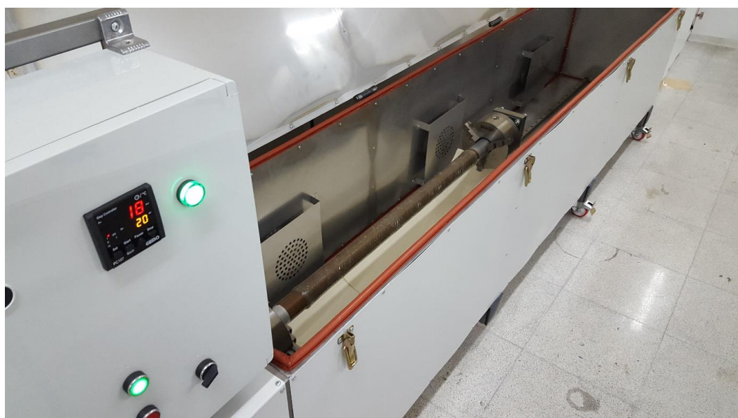
Figure 3.19. Curing oven with rotating shaft.
