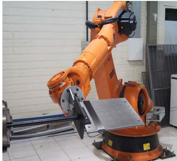
Figure 2.29. Manufacturing of composite plate by filament winding technique.
