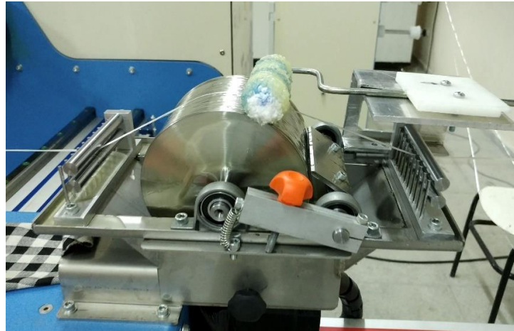
Figure 3.18. Resin bath for filament winding manufacturing.
