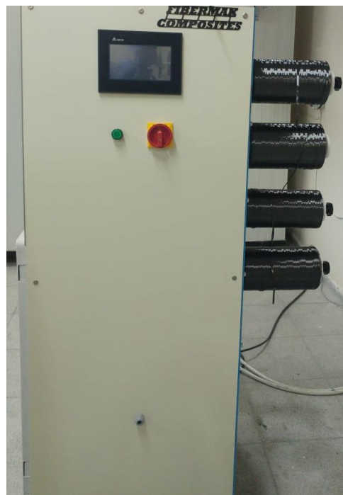
Figure 3.17. Fiber tensioner system for filament winding manufacturing.
