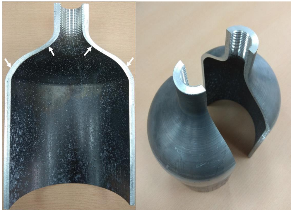
Figure 3. 24. Cross section of the manufactured liners used within the study.
