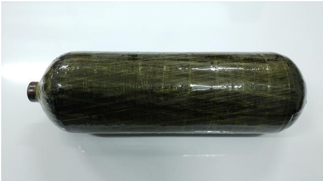
Figure 3.21. A steel liner-based carbon/glass fiber hybrid composite tank after curing.
