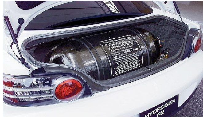
Figure 1.2. Placement of a Type III hydrogen tank in a vehicle
