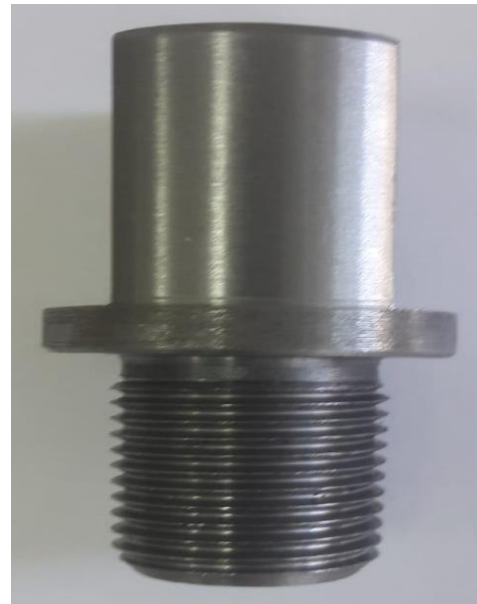
Figure 3.27. (a) Technical drawing and (b) photograph of adapter for steel-based tank.
