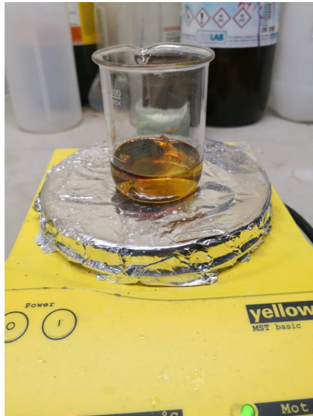
Figure 3.6. Carbon/epoxy specimen in an acid solution during the matrix digestion test.
