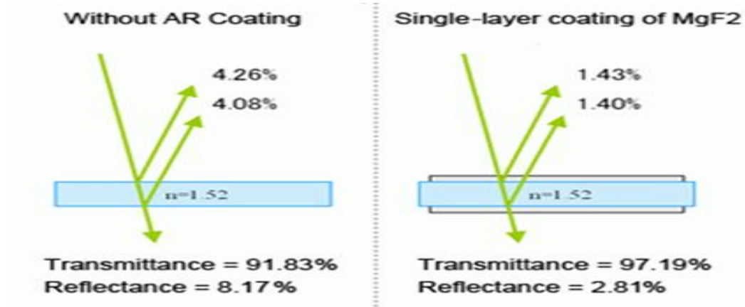
Figure 2.2. Spreading light rays onto the substrate through a single-layer film ( n_s > n ). (Source: Raut, et al. 2011).
