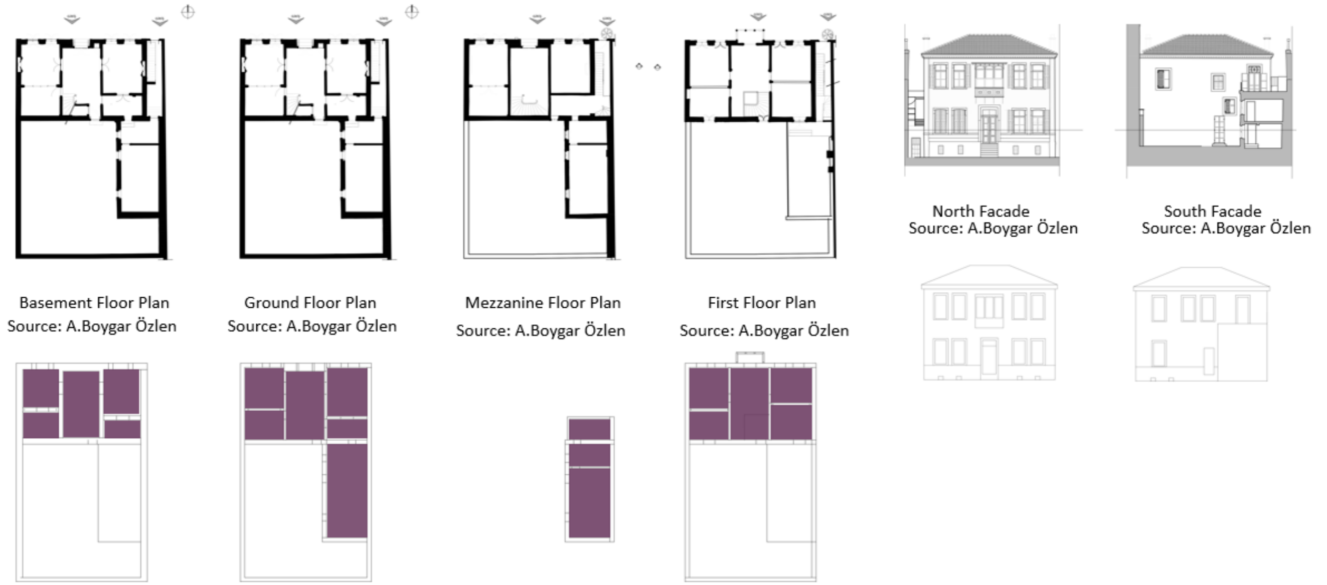
Figure D. 4. Floor Plans and Facades of İzmir Houses Sample with Two Story and Central Hall Plan Type (Source: Boygar,Ö., Restoration Project; İzmir Metropolitan Municipality Archive)
