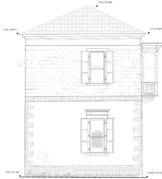
Figure 3.14. East facade of the house in Basmane (Source: Düzalan and Açı, 2016)
