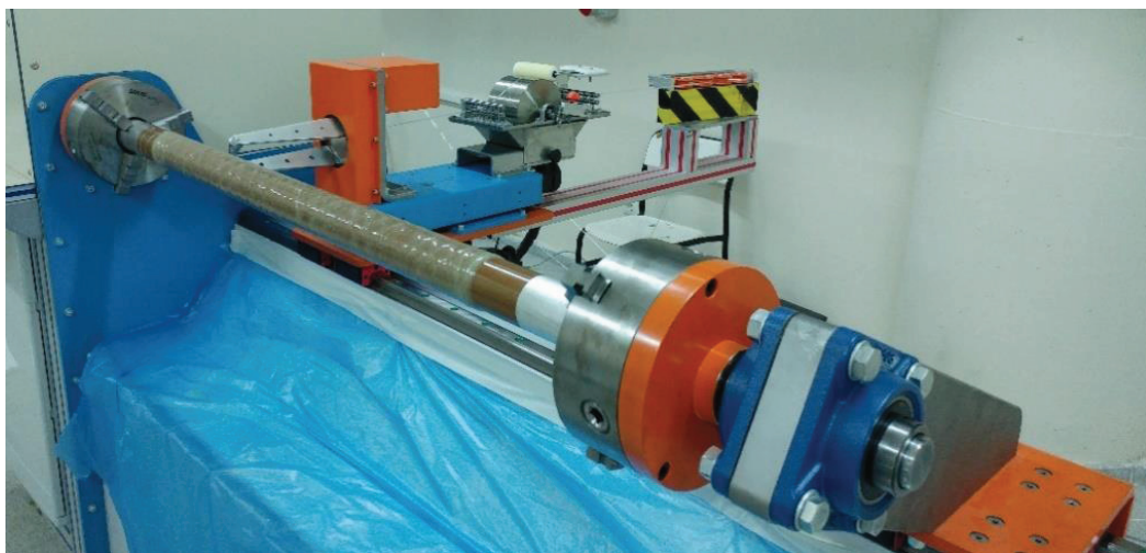
Figure 3.5. Filament winding process of fully glass composite tube
