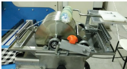
Figure 3.3. Photo of resin bath during the manufacturing of glass fiber reinforced composite tube
