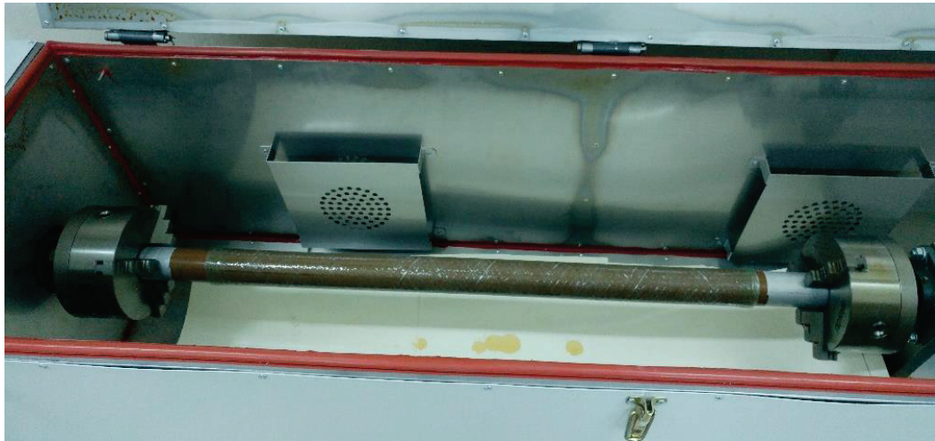
Figure 3.6. Specialized curing oven for filament winding
