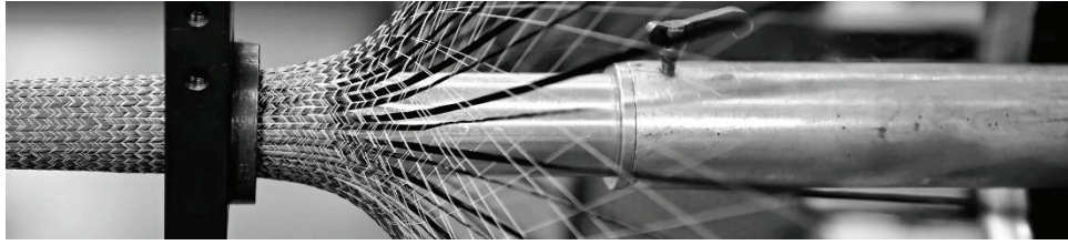
Figure 1.10. Photograph of the pullbraiding process by using carbon fibers
