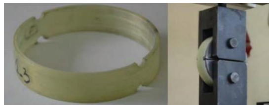
Figure 2.1. Glass fiber composite ring sample and split-disk test fixture with sample (Source: Srebrenkoska, Risteska, and Mijajlovikj 2015)
