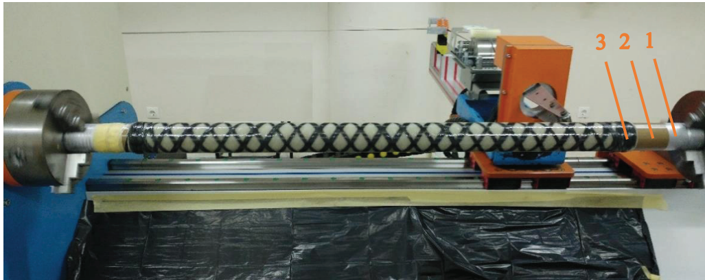
Figure 3.4. Filament winding process of hybrid composite tube
