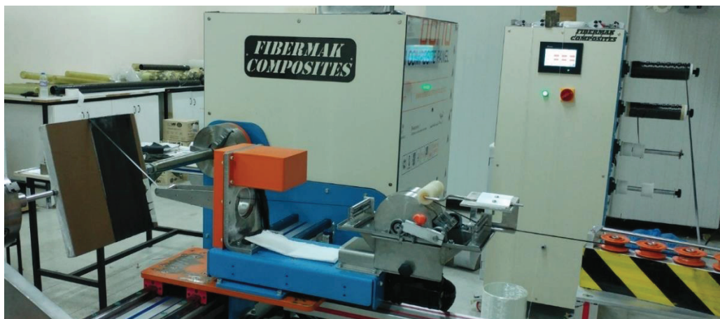
Figure 3.2. Filament winding machine and tensioner with carbon fiber roving
