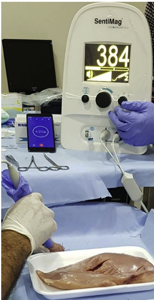
Figure 3 Measuring the Activity With SentiMag in the Specimen
