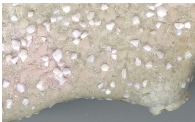
Figure 1. Photograph of corroded refractory brick (GS-M)
