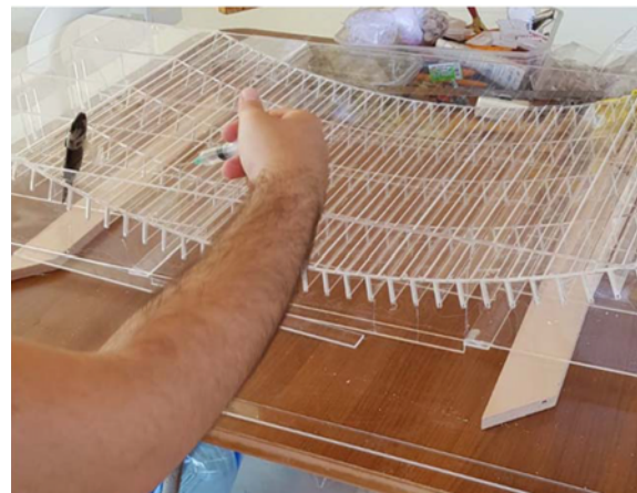
Fig. 3. Manufacturing of the Coanda Intake
