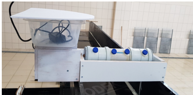
Fig. 6. Sediment Feeding System Used in the Experiments
