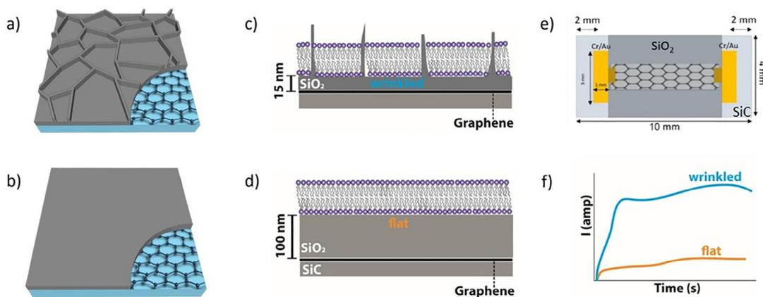
**Fig. 1.** Schematic representation of wrinkle a) and flat b) surface after SiO<sub>2</sub> thin film deposition on epitaxial graphene grown SiC substrate with TE and PED, respectively. Schematic figure of lipid bilayer formation on wrinkled c) and flat d) SiO<sub>2</sub> surface. e) Schematic representation of GFET device and f) time dependent current difference of wrinkled and flat SiO<sub>2</sub> surface after lipid adsorption.
