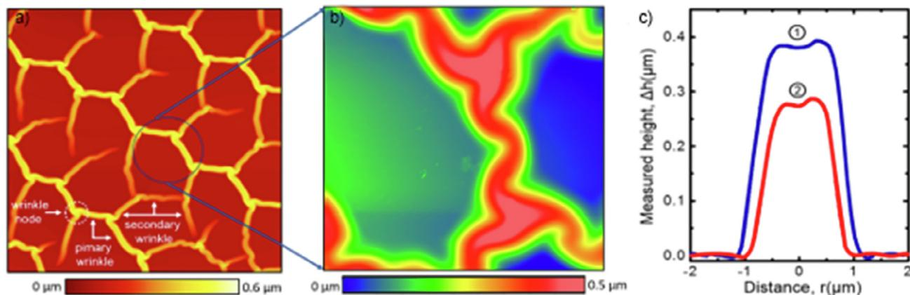
**Fig. 2.** a) 50 × 50 μm<sup>2</sup> AFM topography image of TE deposited SiO<sub>2</sub> wrinkle network on epitaxial graphene b) 10 × 10 μm<sup>2</sup> AFM topography image of localized height protrusions c) Cross-sectional line profiles of primary and secondary wrinkles (1 and 2 indicates the primary and secondary wrinkles, respectively).
