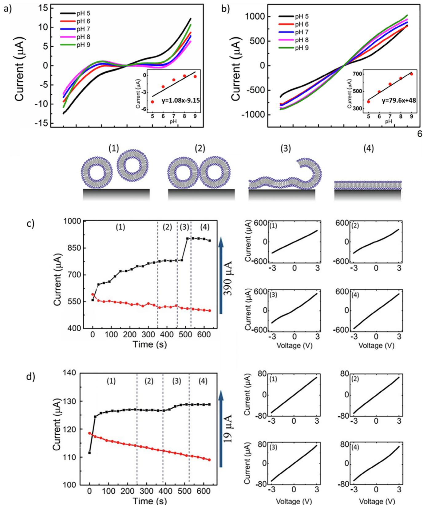
**Fig. 3.** I-V characteristics of pH dependence of a) flat interfaced-GFET b) wrinkle interfaced-GFET. Insets show linear fitting of current versus pH values of flat interfaced-GFET and wrinkle interfaced-GFET, respectively. Time dependent current measurements of lipid vesicle adsorption characteristics of c) wrinkle and d) flat interfaced-GFET surface and their I-V measurements of corresponding parts between  $-3\text{V}$  and  $3\text{V}$  bias.
