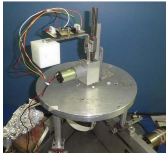
Figure 3 An experimental setup of CaPaMan as earthquake simulator at LARM with a slider-crank mechanism.
