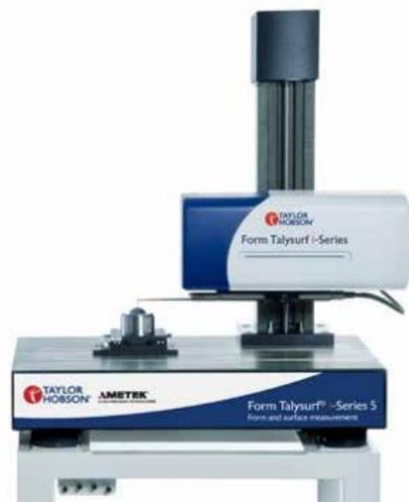
Figure 2.8 Surface roughness measurement instrument Form Talysurf120 (Source: [26])
